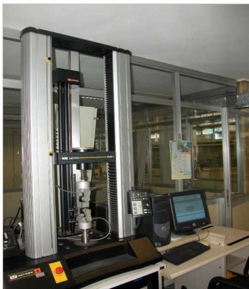
Fig. 2: Tensor check Instron Mod. 5566
